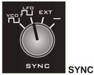
VCO2 only. This switch routes a sync signal to VCO2. Oscillator sync is where a master signal (selected by the switch) will reset the waveform of a slave signal (VCO2 in this case) each time the master waveform starts a new cycle.
